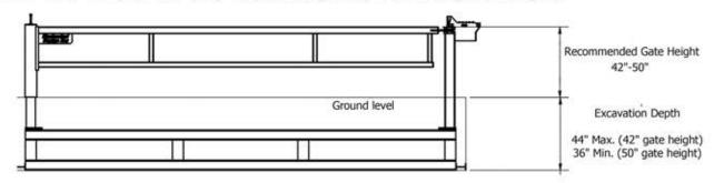
3 > PLACE GATE & LEVEL: Use of string line, laser level, etc is recommended. Backfil with gravel to level as needed.
